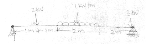
b) Draw shear force and bending moment diagrams (10M) neatly.
